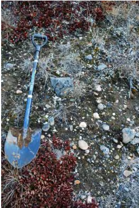
Photo A-16 Texture of glaciofluvial material at Borrow Source 172
