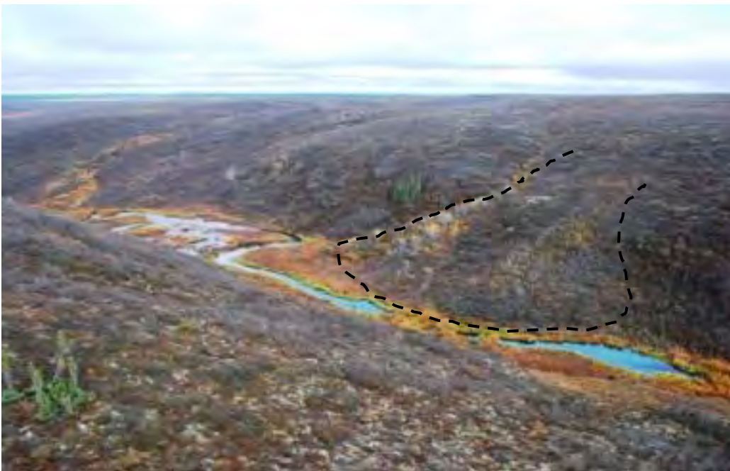
Photo A-10 Old stabilized slide (dashed line) along the eastern bank of a stream at Borrow Source 2.45 (looking northeast)
