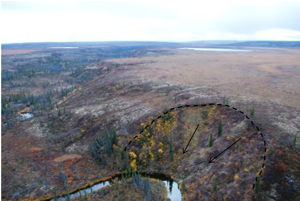
Photo A-14 Active slumping (dashed line) along the edge of a terrace at Borrow Source 325
