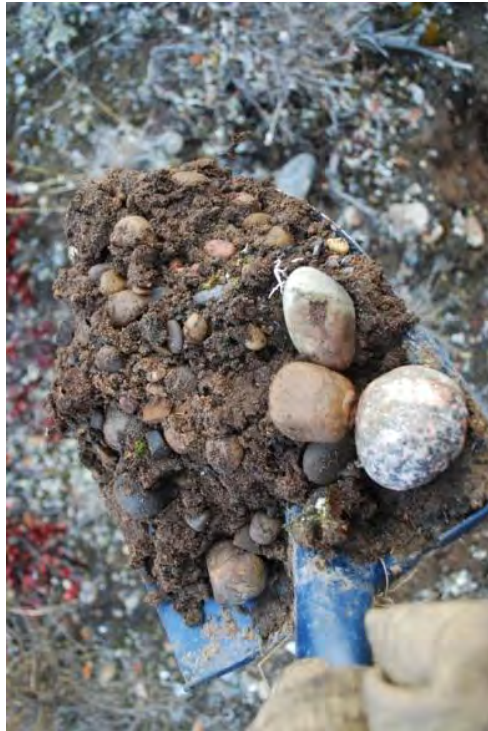
Photo A-16 Texture of glaciofluvial material at Borrow Source 172
