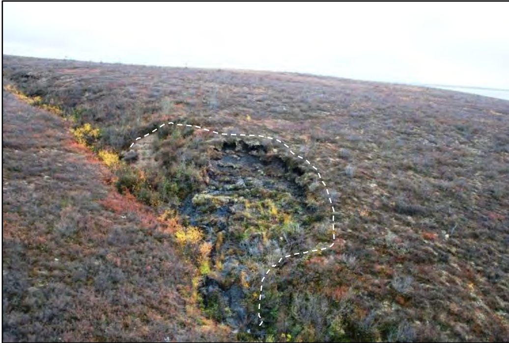
Photo A-9 Small active-layer detachment failure next to a gully at Borrow Source 2.45
