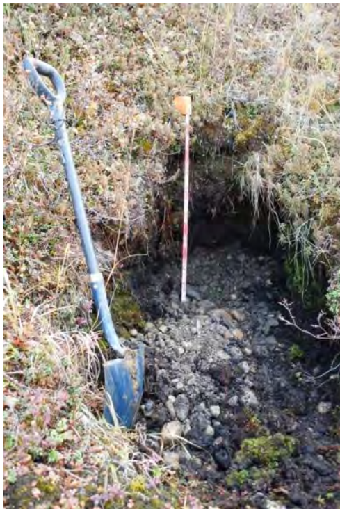
Photo A-8 Coarse-grained glaciofluvial material at Borrow Source 2.45
