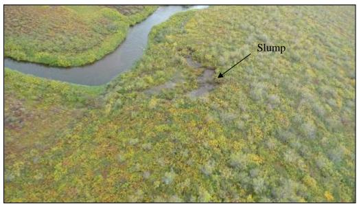
Figure 8 Small, active slump on a cutbank of Zed Creek, downstream of the proposed highway crossing.
