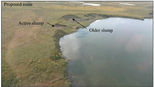
Figure 9 Active and revegetated slumps on a lake-shore next to the proposed route.
